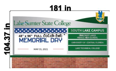
Lake Sumter State College - Internally Illuminated Channel Letters 4x8 Double Sided Full Color EMC Back Illuminated Negative Cut Panels Stone to be done by others. Sign will have required Hardy Board needed for mounting.
